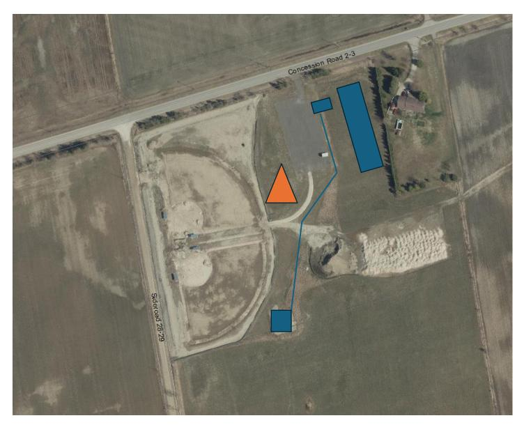
Boxes and lines drawn on photo indicate Well 5 infrastructure – water lines, pumphouse, treatment lines. Nothing can be built on top of buried infrastructure. Road crossings over water lines will require culverts/other infrastructure over the lines.
